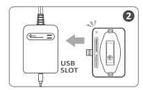
Connect the Charging Dock to USB connector on the Battery Charger. The light indication on the Charging Dock will be shown still red.
