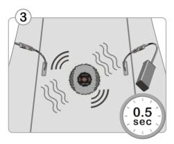
Once both ends are connected, a vibration signal (0.5 sec.) will indicate that the learning mode has been activated.
