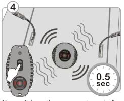
Now switch on the new remote controller, you can feel the vibration (1.5 sec.) Correspondent with the switch in each setting. Unplug the match pin.
