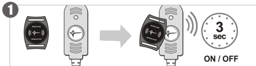
Turn on and off the Thermalution Blue Grade by simply placing the CPS panel next to the CPS controller and holding them together for 3 seconds. The indication lights on the CPS controller will show the power status of the undersuit.
